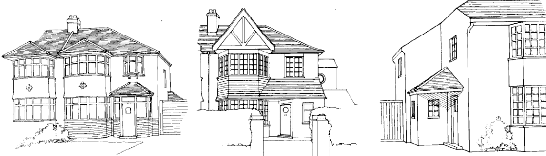
Picture: Examples of angled porches which blend in with the bay windows.
